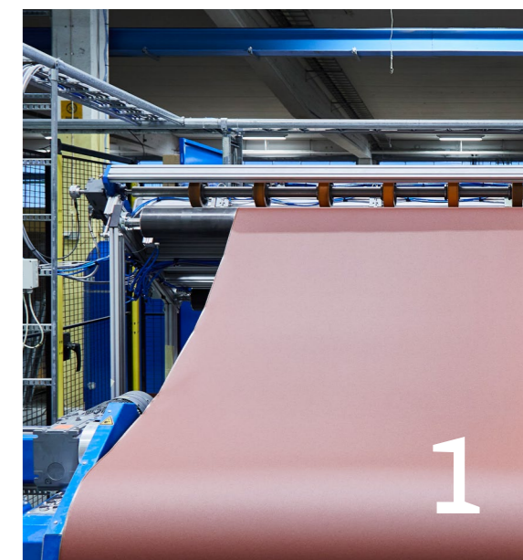
Feeding the automatic rewinder
